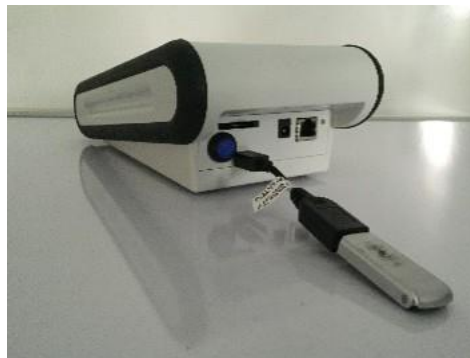
USB (type A) adapter to USB (type A) device (USB flash drive shown)
